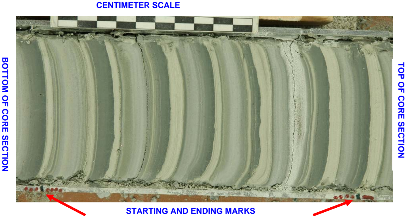
Figure 1. High resolution image of core section from core site at Claremont Junction, New Hampshire.
