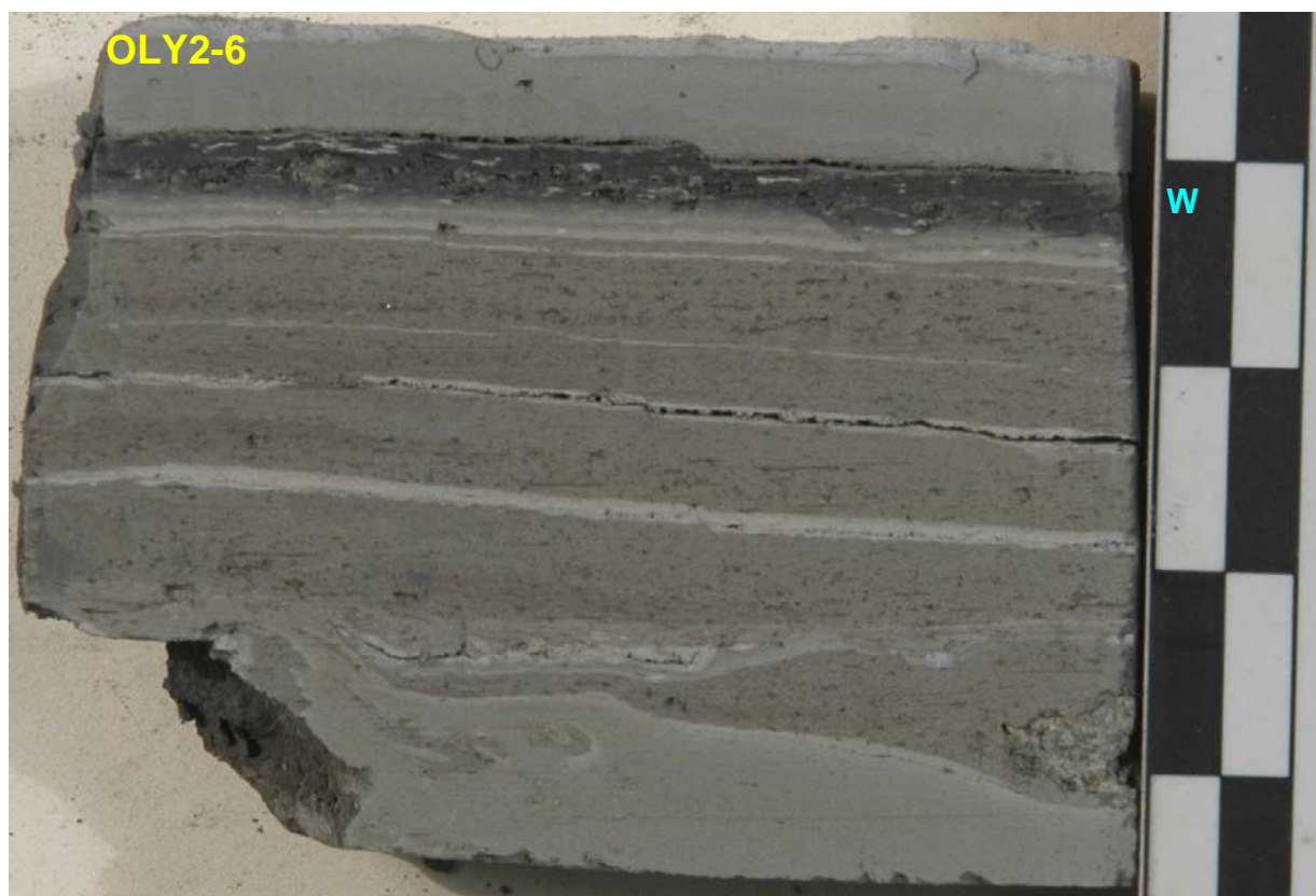
Note low-angle faults and warped bedding in OLY2-4 and contorted layers due to mass flow at base of OLY2-6.
