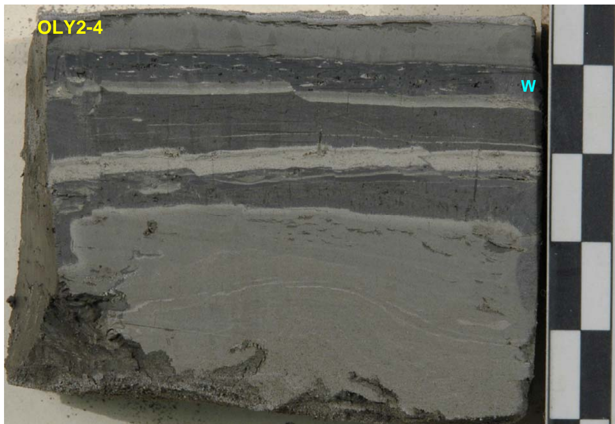
Note low-angle faults and warped bedding in OLY2-4 and contorted layers due to mass flow at base of OLY2-6.
